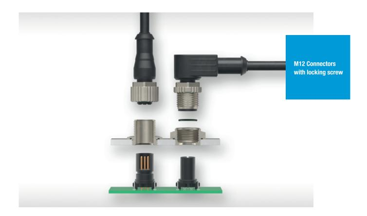
Since the 1980s, M8/M12 connectors have been used in sensor technology and industrial automation devices. The connectors were developed for higher protection classes such as IP65 or IP67. The mating face is coded and standardized so that end customers can use cables from different manufacturers.
